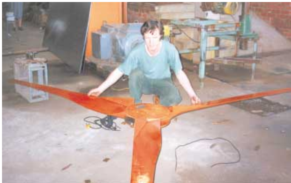
Hugh balancing a set of wooden blades for an African machine.
