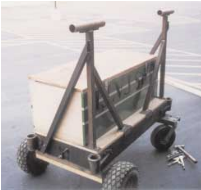
The battery box in position. Sturdy uprights are braced to hold weight and resist wind forces on the PV rack.
