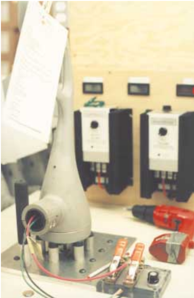
Every AIR is load tested to rated RPM. Intake of the wind tunnel.
