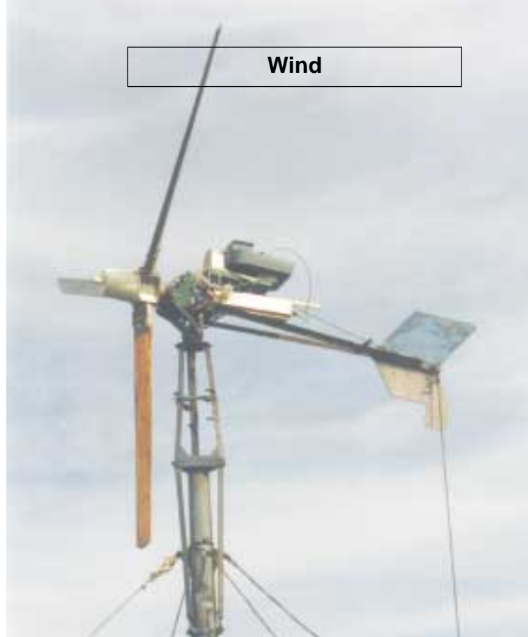
Another home-built gearbox machine. This one also has pitch control and a synchronous alternator.
