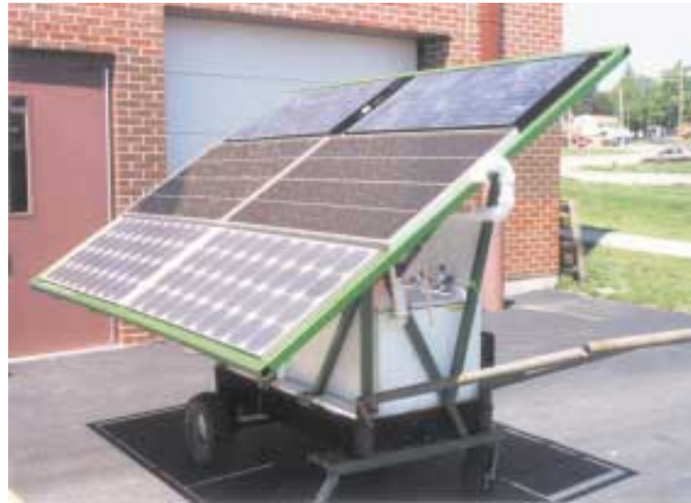
The Rolling PV Workstation with 350 watts of PV deployed and soaking up the sun. Two Solarex MSX 64 poly-crystalline panels on top, two Solarex MST 40 LV thin film panels in the middle, and two Siemens SP75 single crystal panels on the bottom.
