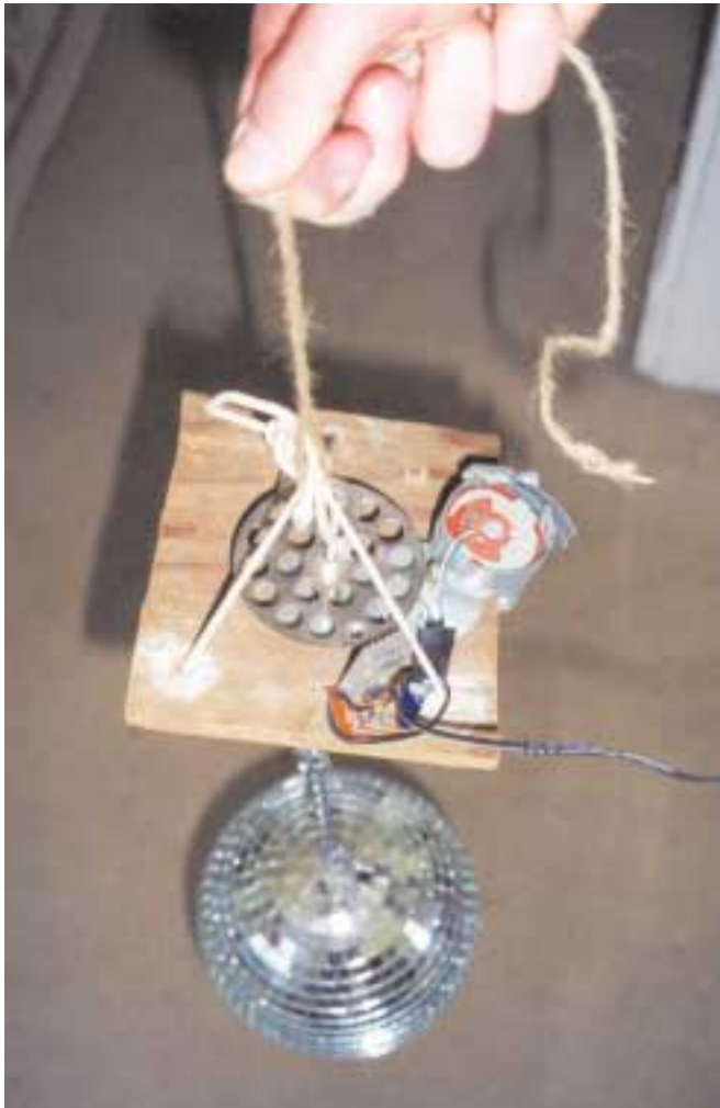
Drive assembly for Y2KdB. The small circuit board holds the circuit shown in the schematic diagram below. Notice the generous heatsink on the LM7805 chip. The components are fixed onto a scrap piece of plywood, using hose clamps, hemp twine, and old clothesline.
