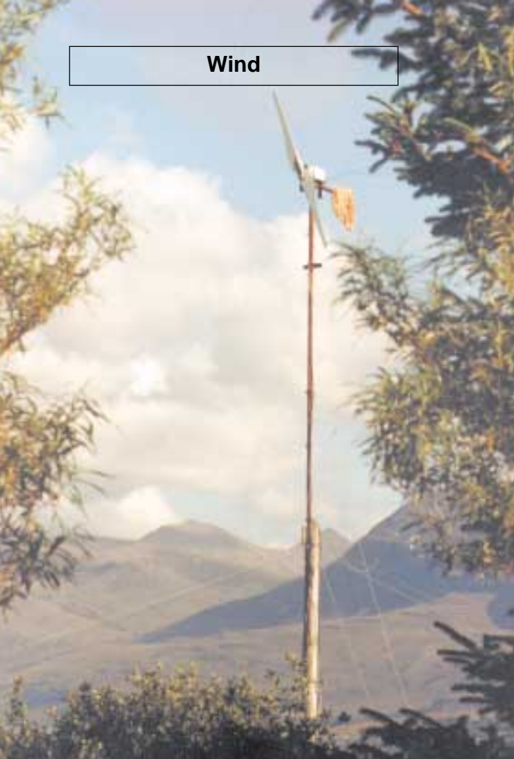
A battery charging wind turbine built by Hugh on Scoraig. The dynamo (generator) came from a bus.
