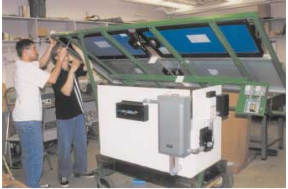
Teamwork: Vance and Mark attaching the PV panels to the rack, taking care not to overtighten the bolts or strike the panels.
