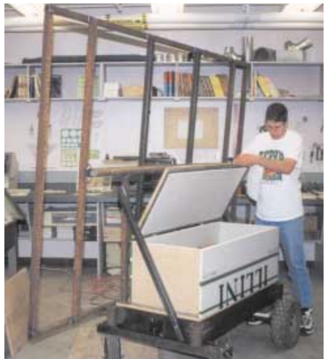
A 6 by 8 foot (1.8 x 2.4 m) PV rack made out of 1 1/2 inch (38 mm) square tubing. Vance inspects the battery box.
