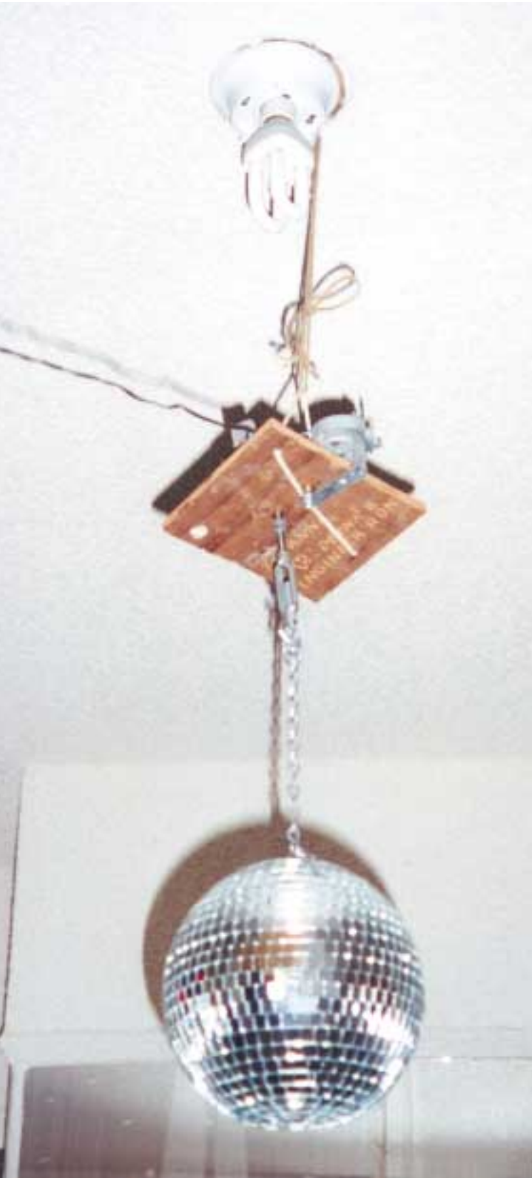
The Y2KdB ready for action. Using string or baling wire, the Y2KdB can be mounted on an existing ceiling light socket or lightbulb. Turn off the circuit breaker first!
