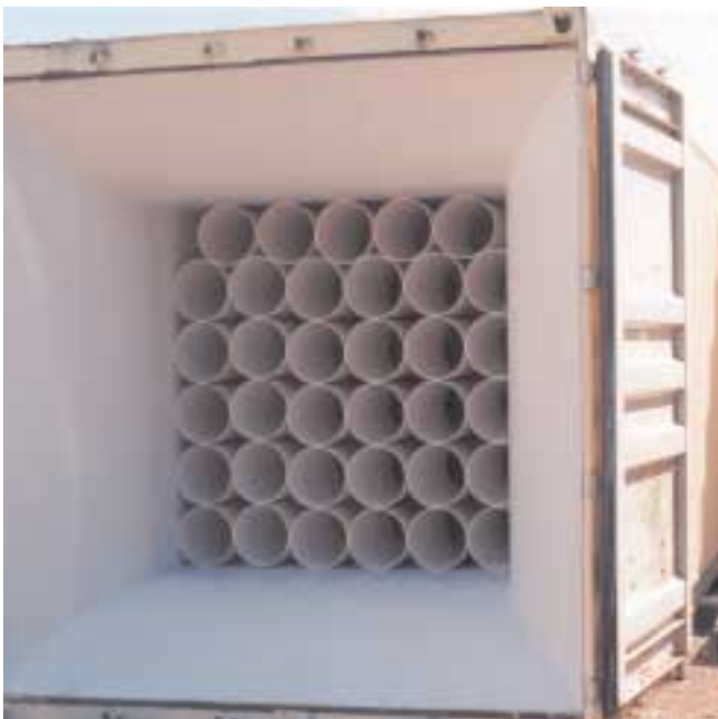
Every AIR is load tested to rated RPM. Intake of the wind tunnel.
